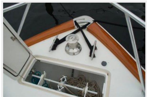
Winlass, Anchor locker
