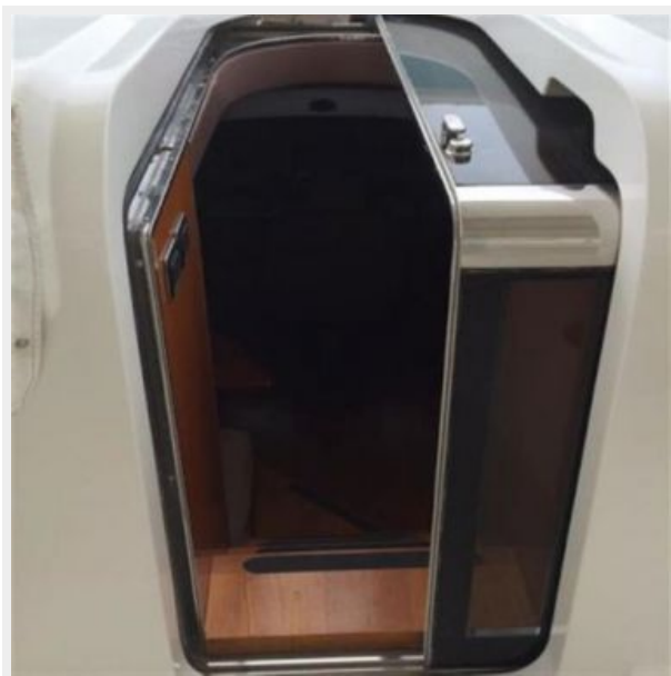
Sliding hatch to Flybridge
