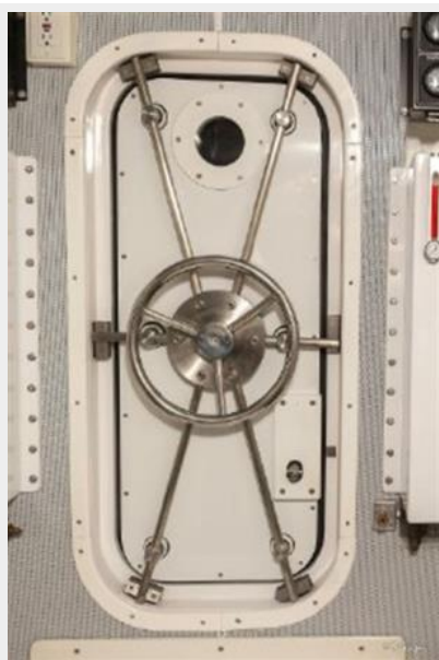
Water Tight Door
