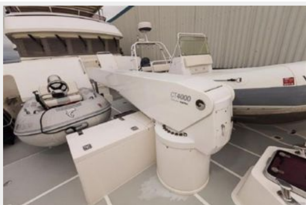
Boat Deck Crane
