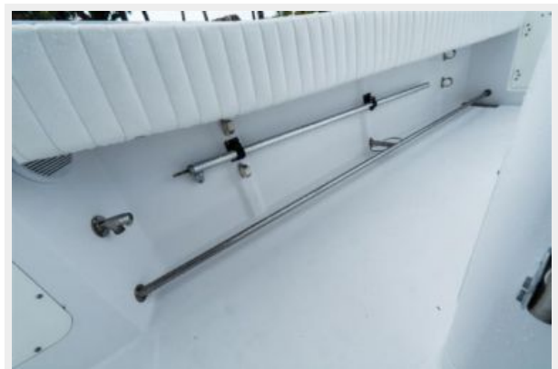
Cockpit Rod Storage/Toe Rail STBD
