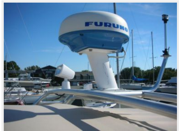
30' Mainship Radar dome
