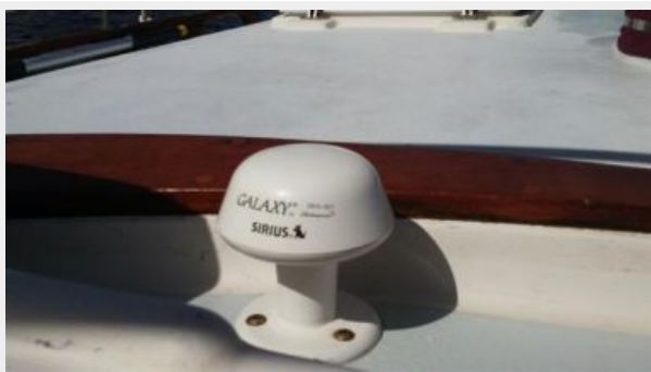
Sirius weather system antenna
