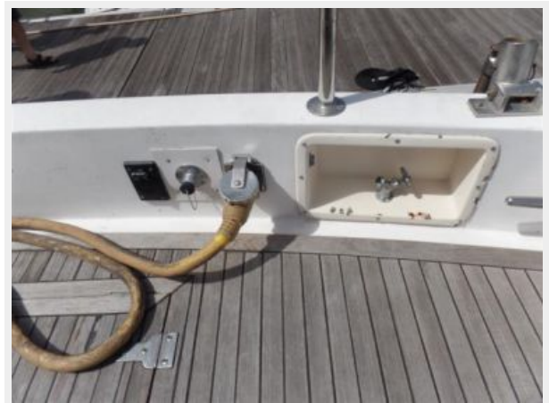
Transom shore power and water.JPG
