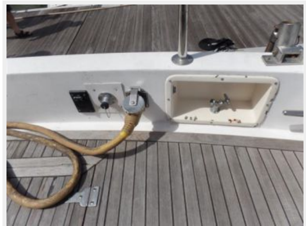
Transom shore power and water.JPG
