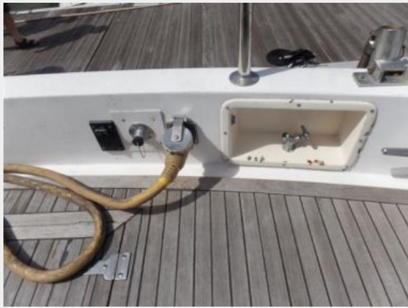
Transom shore power and water.JPG
