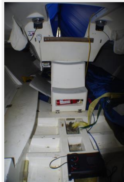
Companionway/stairs/engine box and showing the keel floors
