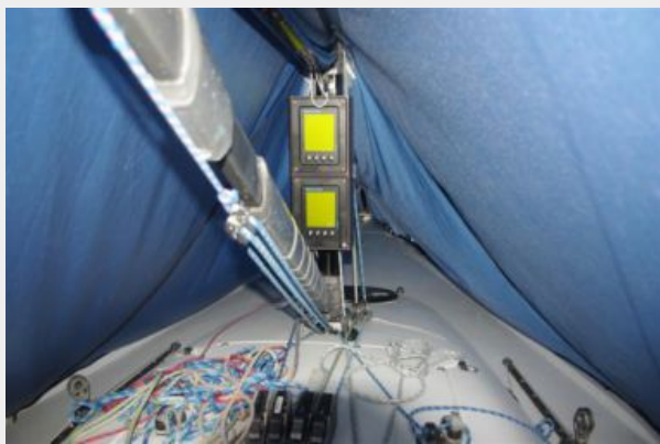
Vang, control lines and heads up displays
