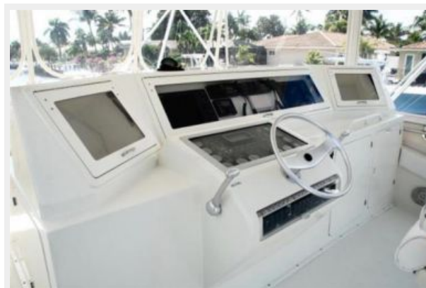
Flybridge Helm Console
