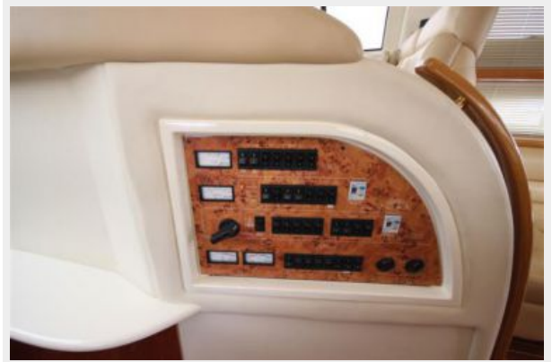
Main Distribution Panel
