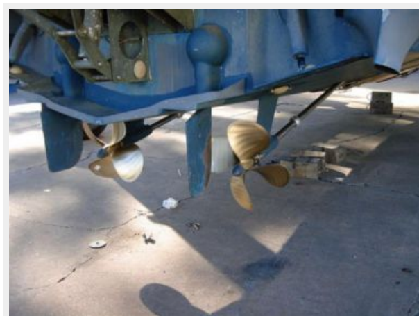
Props, shafts struts and attachments for Sealift
