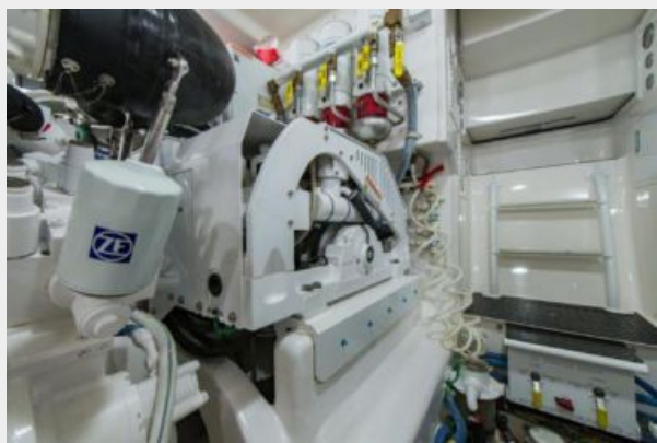
Sea Keeper GyroStabilizer
