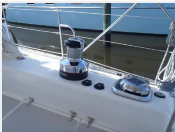
Stbd Electric Primary Winch
