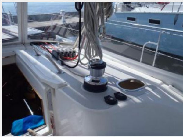
Stbd Electric Halyard Winch
