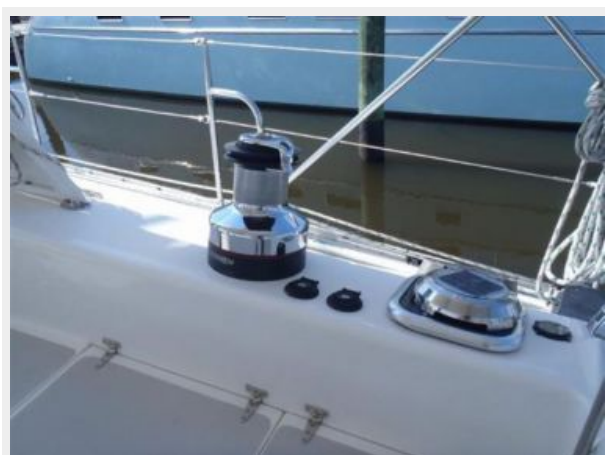
Stbd Electric Primary Winch
