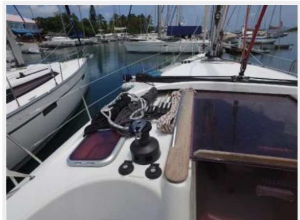
Port Rope Clutches and Electric Winch
