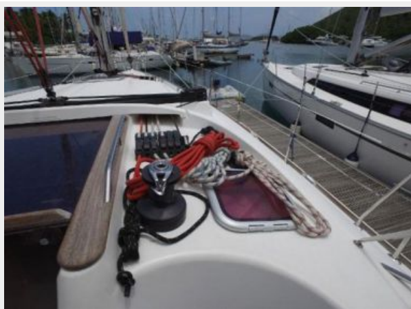
Port Rope Clutches and Electric Winch
