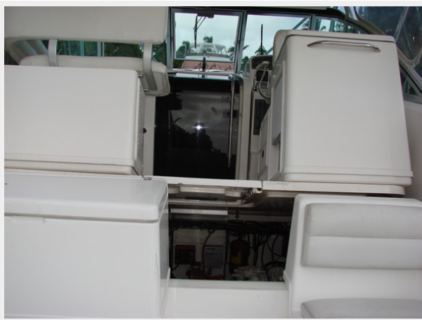
Entire Helm Sole with Seating on Electric Lift Access to Engines
