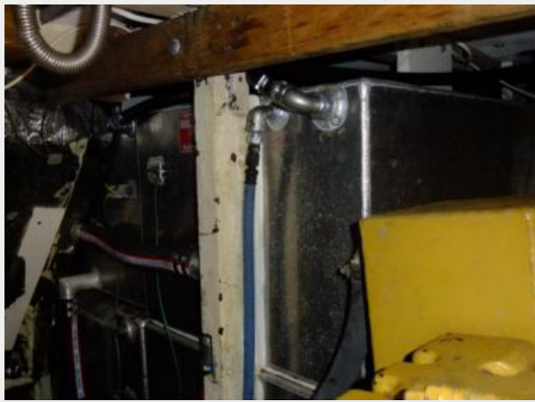
Grand Banks 42 - Engine Room New Fuel Tank Port Side
