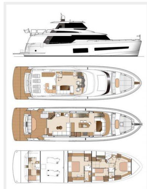
Enclosed Bridge Layout
