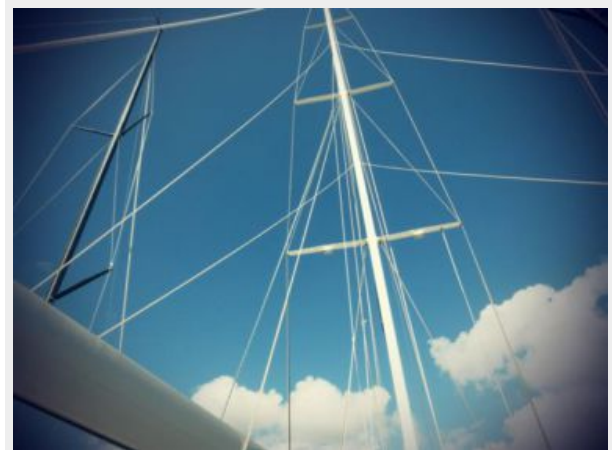
C & C 41 Keel Stepped Mast w/ Running Back Stays
