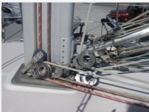
Mast Base w/ running rigging
