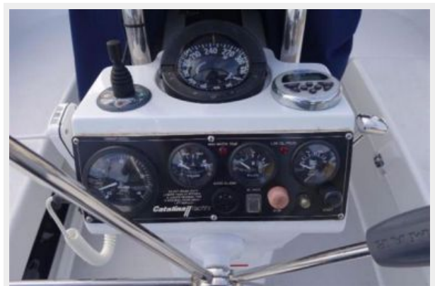
Gauges and Bow Thruster Control
