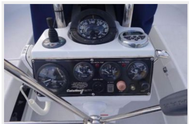
Gauges and Bow Thruster Control
