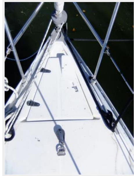
Beneteau 285 - Forwadr Deck Anchor Locker
