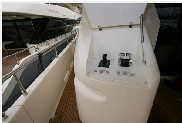
3rd engine control - bow stern thruster control
