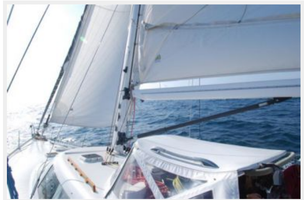
All Line Sheets Lead Back to Cockpit
