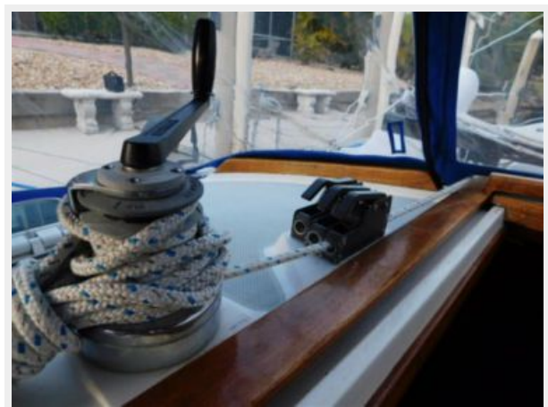
21 42' Catalina self tailing winch and line clutch
