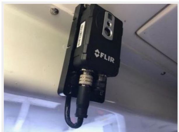
Engine Room Camera
