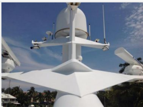
MAST - Sat Com Dome
