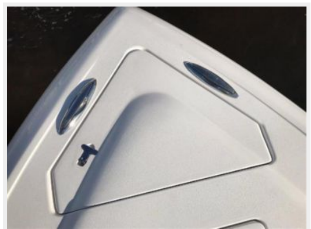
327 Intrepid | Windlass anchor hatch
