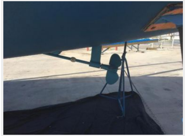
Feathering Max prop with Shark shaft
