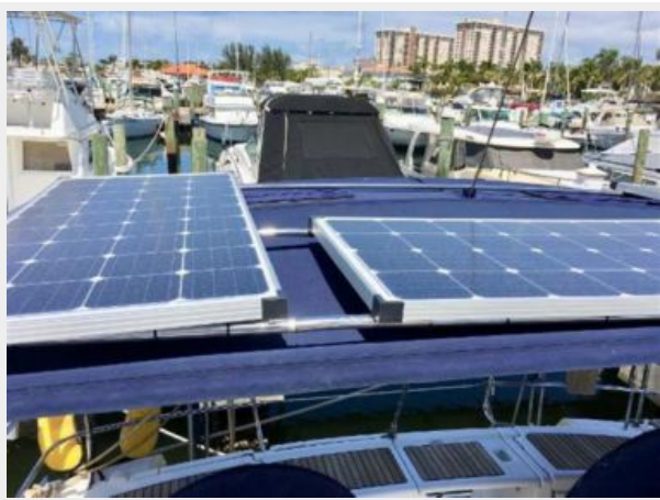
Solar panels on a rack over the Bimini frame 480 Watts new in 2018
