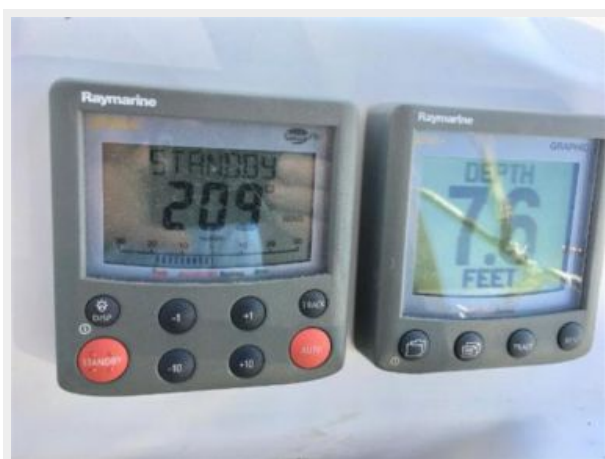
Raymarine Autopilot display and ST60 Multi on starboard side steering station
