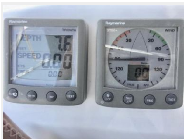
Raymarine ST60 tridata and wind on port side steering station
