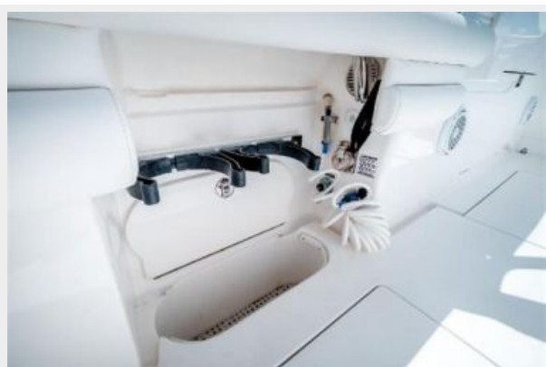
Port/Stbd Dive Tank Storage
