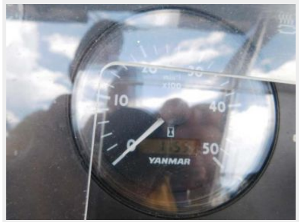
Yanmar Tach and Hour Gauge
