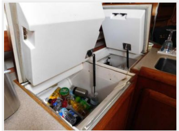
Refrigeration with Gas Shock Assisted Lids
