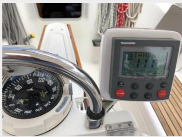
Plastimo steering compass and Raymarine ST6001 control at helm
