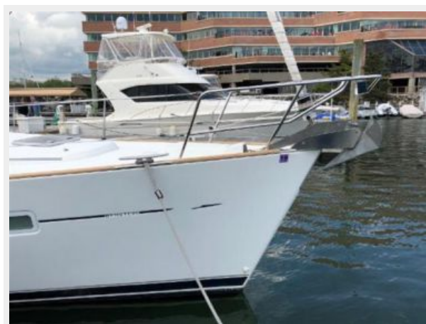
Starboard bow with 44 LBS Delta anchor detail
