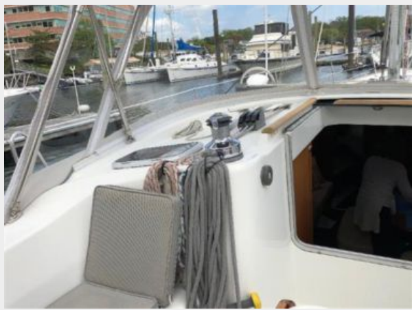
Port side electric maneuvering winch
