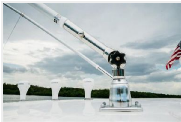
18' Taco Telescoping outrigger poles
