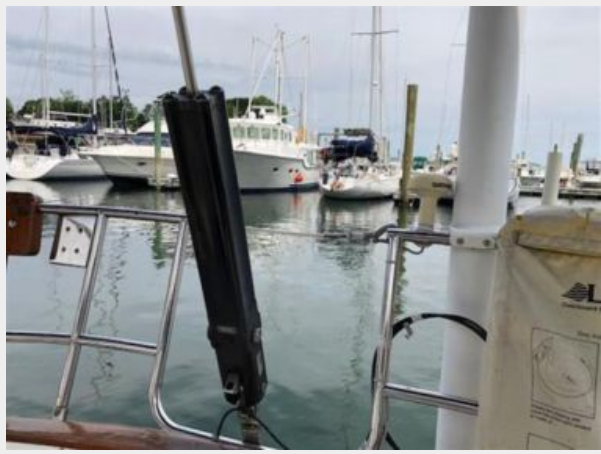
Navtec Hydraulic backstay adjuster
