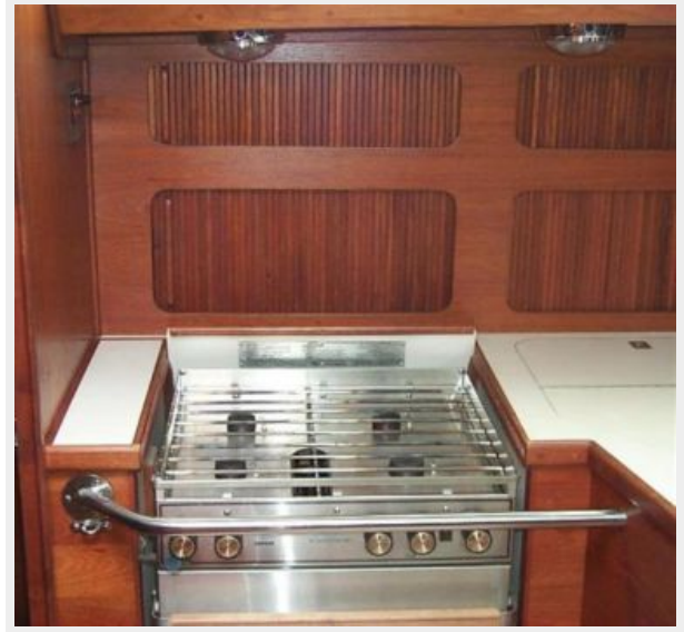
Four burner stove with oven
