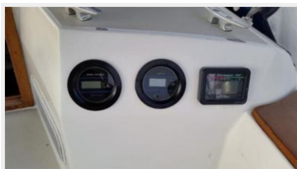
Depth and speed on the starboard bulkhead
