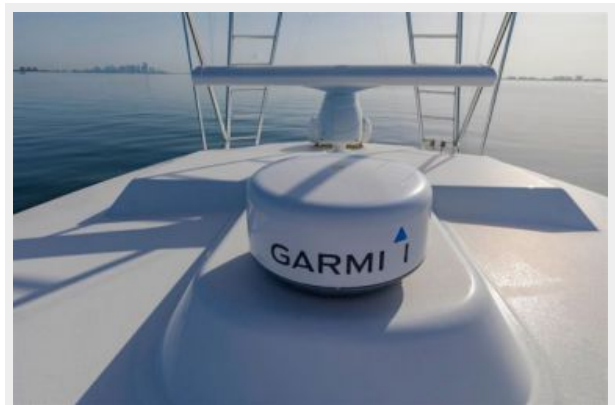
Dual Radar Units
