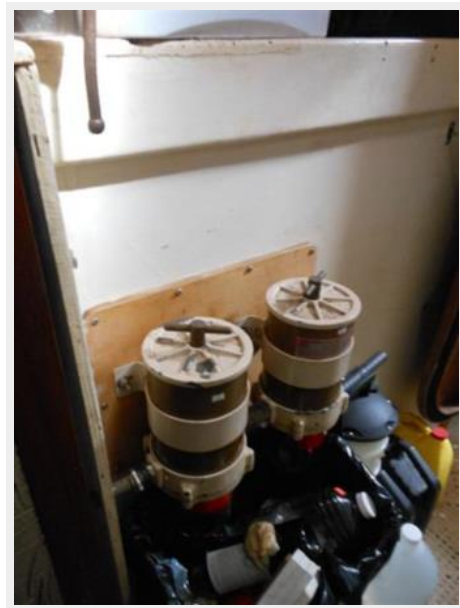
Dual Racor fuel filters outside ER
