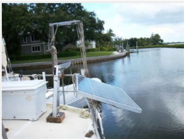
80W Solar Panel & Custom Motor Hoist
