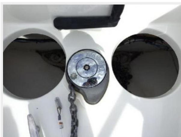
Fender Storage - Anchor Locker
