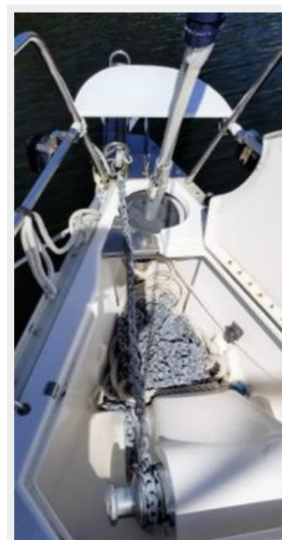
Chain Locker with windlass
