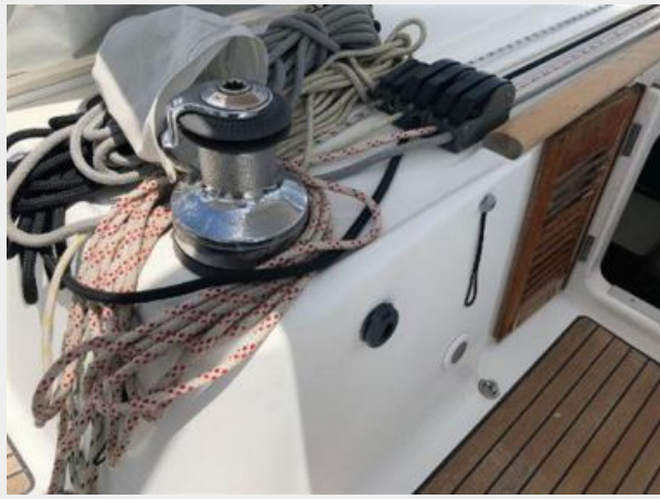
Port side electric maneuvering winch
