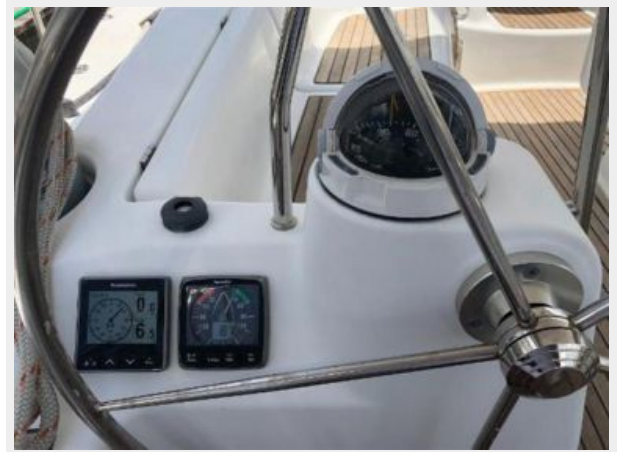
Port side steering station with i70 Raymarine Multi and i60 Wind
