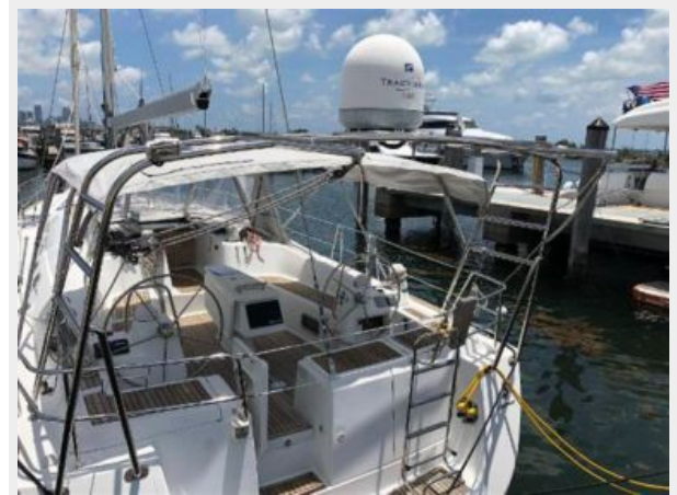
Arch with KVH satellite TV antenna
