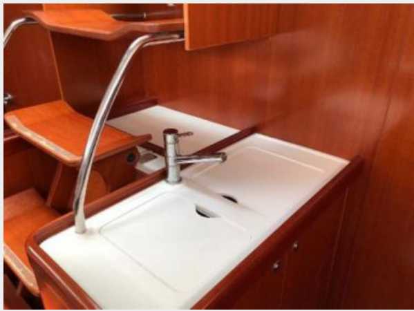
Galley zincs with covers for more working space
