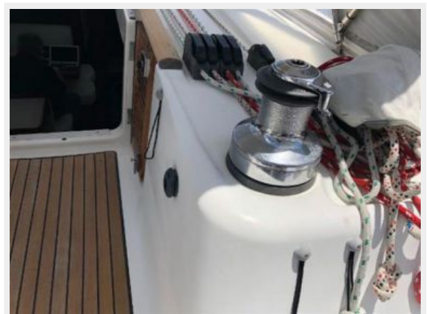
Starboard electric maneuvering winch
