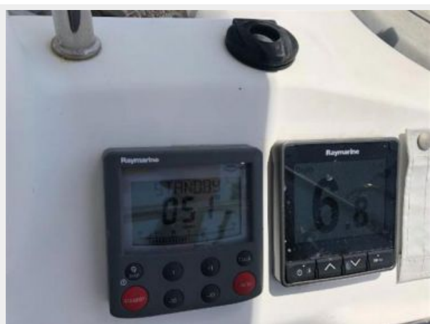
Starboard steering station i70 Multi and auto pilot
