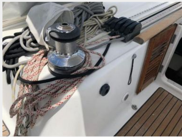
Port side electric maneuvering winch
