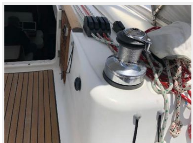
Starboard electric maneuvering winch
