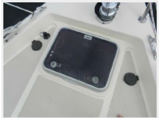
Bow Locker, Salt Water wash-down, foot switches for windlass
