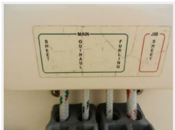
All sail controls from aft cockpit...
