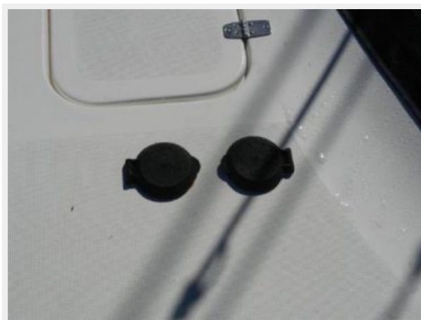
Foot switches for windlass
