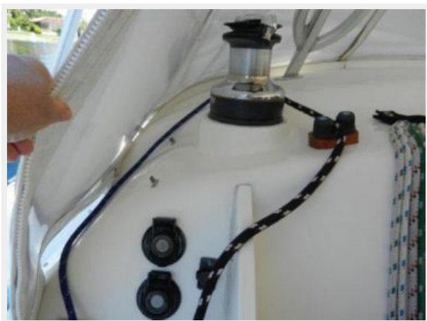
Electric winch for all sail controls
