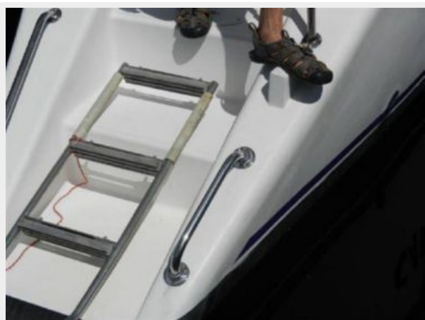
Custom boarding steps on both hulls transoms
