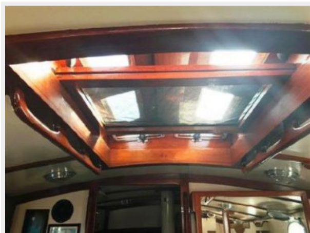
Butterfly Hatch & Hand Rails_Interior
