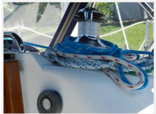
Electric Winch on cabin top
